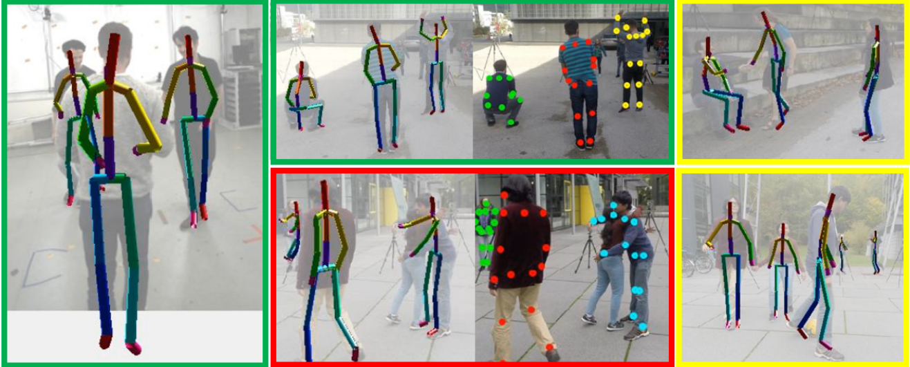
Figure 9. Visualization of predictions from our method for frames from our multi-person 3D pose test set. Our method can handle strong occlusions (green box on the left), but occlusions where neck and pelvis detections both fail result in people not being detected (red box). Mild limb pose failures are shown on the right (yellow boxes).
