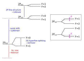
Fig. 2. The 2S and 2P energy levels in the muonic helium-3 ion. The inset on the right displays the shift  $\Delta$  of the 2P levels due to the mixing of levels with same quantum number F, as described in Section 5. The figure is not to scale.
