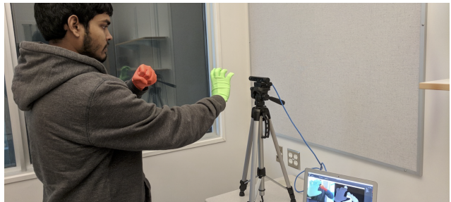
Figure 2. Our dataset is constructed by recording a user performing hand movements wearing a pair of bright colored gloves in front of a depth camera. To the best of our knowledge, our dataset is the first two-hand dataset for hand segmentation.
