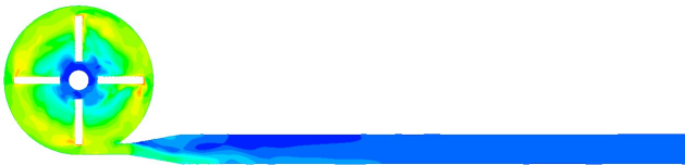
Figure B.13: Velocity at blade passage plane, 6.0 L/min, 3500 rpm
