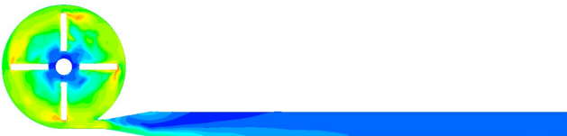
Figure B.14: Velocity at blade passage plane, 7.0 L/min, 3500 rpm
