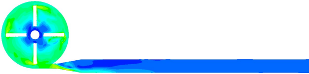
Figure B.12: Velocity at blade passage plane, 6.0 L/min, 2500 rpm
