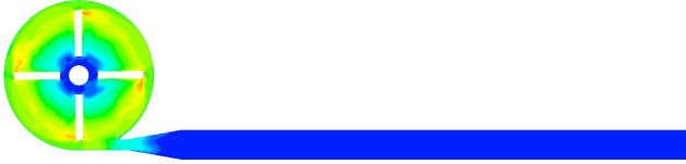
Figure B.10: Velocity at blade passage plane, 2.5 L/min, 3500 rpm
