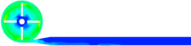
Figure B.9: Velocity at blade passage plane, 2.5 L/min, 2500 rpm
