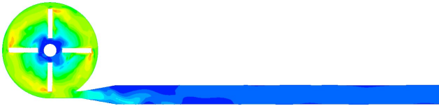
Figure B.11: Velocity at blade passage plane, 4.5 L/min, 3500 rpm
