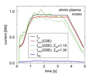
Figure 1: Bootstrap and ohmic current evaluated with 2 different methods and different  $Z_{\text{eff}}$  values.
