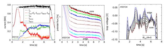
Figure 2: Time traces of the current mixture (left), of the poloidal flux at various flux surfaces from the core to the edge (middle), and of the loop voltage profile (right).
