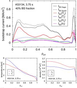
Figure 4: Bootstrap current profile and its constituents calculated with the Sauter formula and a recent modification, and the kinetic profiles used.
