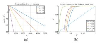
FIG. 7. The figures summarize the results for the  $n \rightarrow 1$  hashing protocol for a single link: Fig. 7a plots the deviation in the output fidelity depending on the number of initial pairs for different initial fidelities. In Fig. 7b the input fidelity versus the output fidelity for varying numbers of initial pairs is shown.
