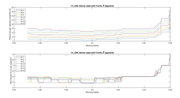
FIG. 12. (top) Plot of the number of elementary Bell pairs needed as a function of the working fidelity for different number of links  $2^N$ . (bottom) Plot of the distribution time as a function of the working fidelity for different number of links  $2^N$  in units of  $t_{\text{segment}}$ .
