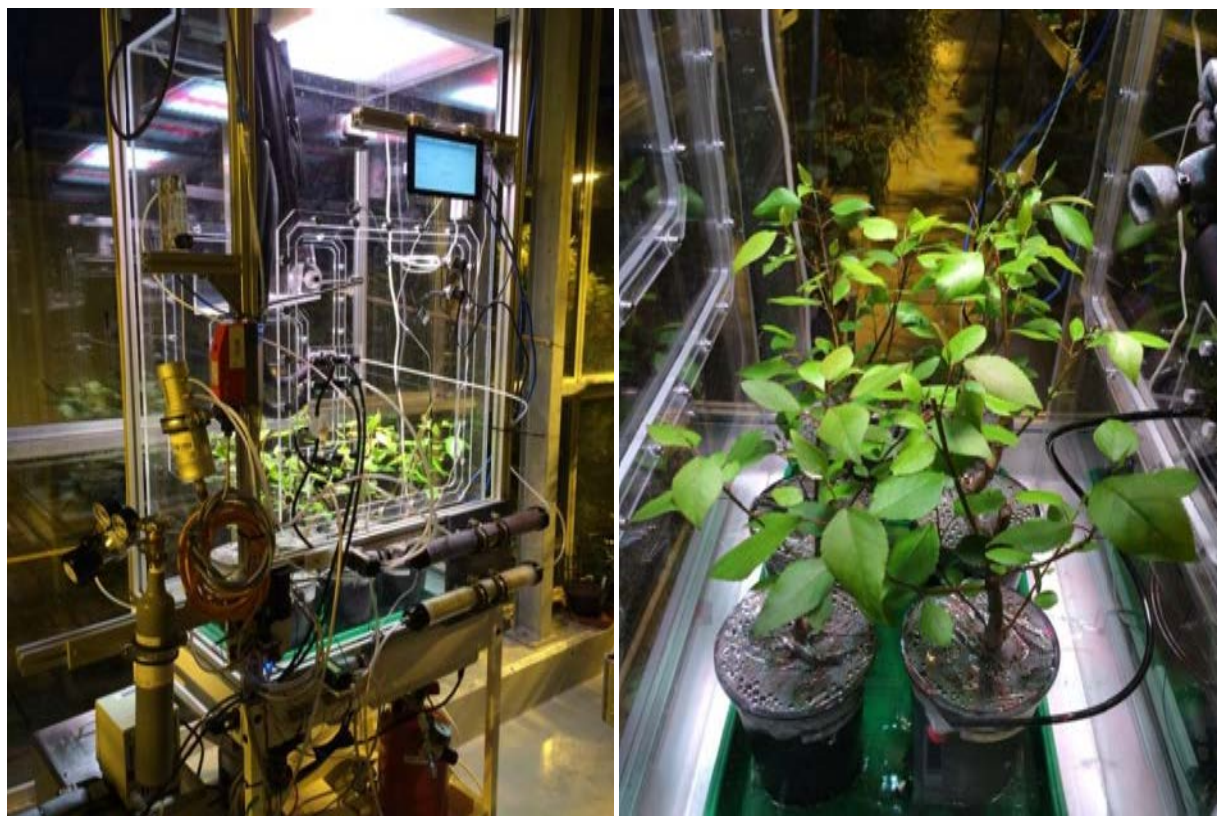
Figure B.1-4 Pictures of the automated growth enclosure for stable isotope ^{13}\text{CO}_2 labeling experiments.
