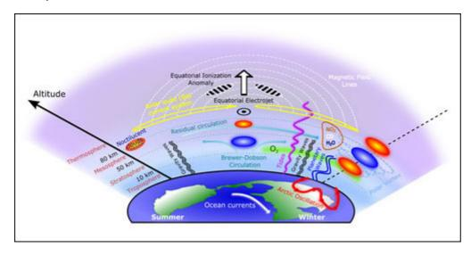
Fig. 1. Schematic of the coupling processes and atmospheric variability that occur during sudden stratospheric warming events. Red and blue circles denote regions of warming and cooling, respectively.
