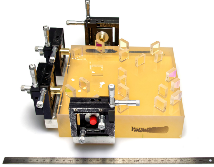
Figure 2. Photograph of the stable interferometer with bonded optical components and fiber injectors for the fiber under test (on the left) and for the delivery fibers. The photo diodes reading out the interferometers are not shown. They were placed next to the Zerodur™ baseplate.
