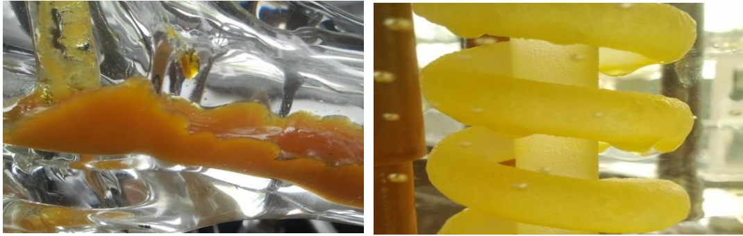
Figure A.7: Solid condensat refined in a SPD plant at high (left) and low (right) evaporation temperatures
