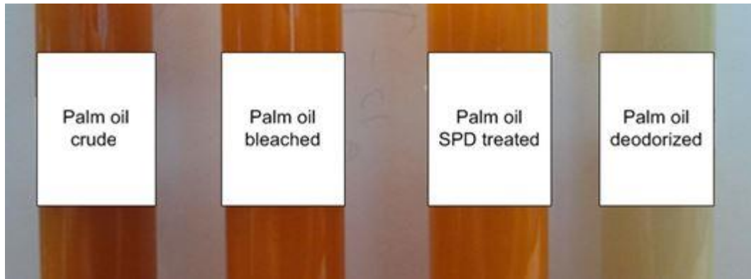
Figure 5.4: Color comparison of palm oil after various refining stages
