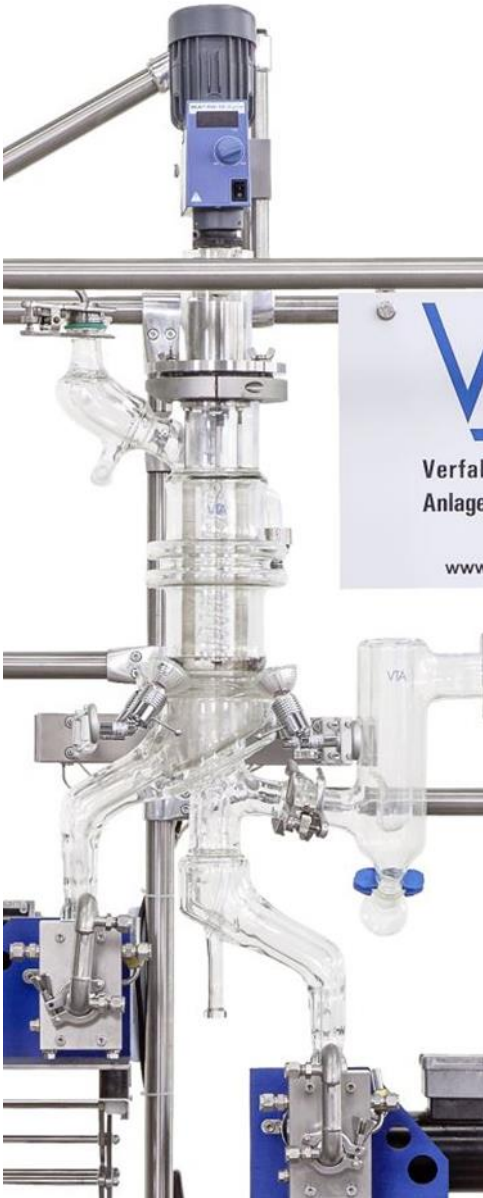
Figure A.2: Technical scale SPD evaporator unit (glas) with integrated spiral condenser
