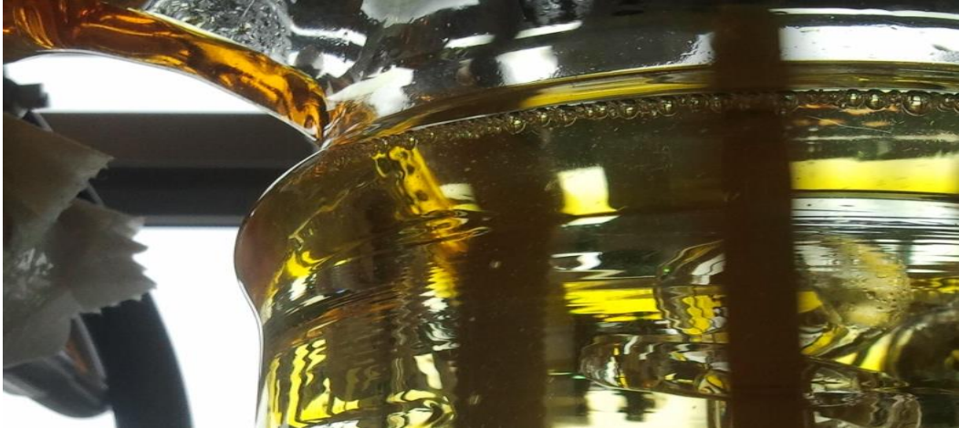
Figure A.6: Layer thickness of palm oil on the the evaporator wall
