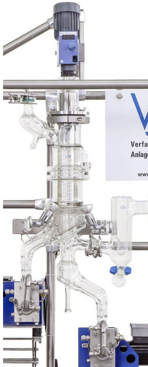
Figure 4.2: Technical scale SPD evaporator unit (glas) with integrated spiral condenser
