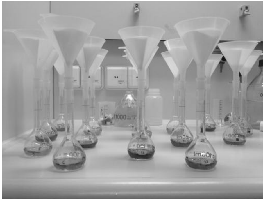
Figure 13: Dithionite extraction at the stage of the second filtering process
