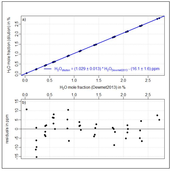
Figure 6: a) Water vapor mole fraction based on the  $CO_2$  dilution method plotted against the water vapor mole fraction measurement of the CRDS analyzer (offset corrected and calibrated according to the comparison against a dew point mirror in 2013) during the fine scan experiment. The corresponding fit is shown in blue. Residuals (difference between water vapor mole fraction based on dilution method and the linear fit) can be seen in plot (b).
