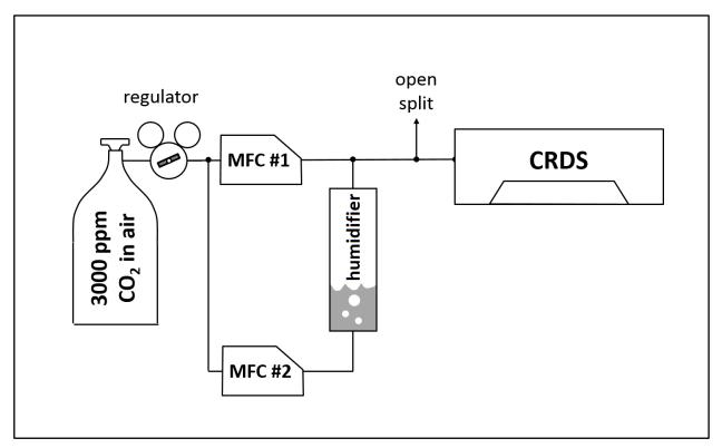
Figure 2: Experimental setup for the water vapor calibration by the CO<sub>2</sub> dilution effect.
