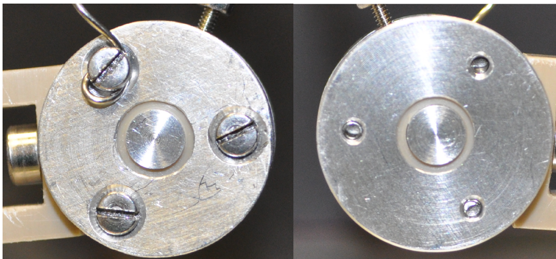
Figure 3.8: Photograph of the bidirectional Faraday cup from both sides.
