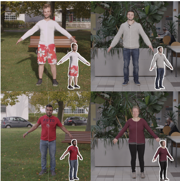
Figure 9. Side-by-side comparison of our reconstructions (right) and the input images (left). As can be seen from the right side, our reconstructions precisely overlay on the input images. The reconstructed models rendered in a side view are shown at bottom right.
