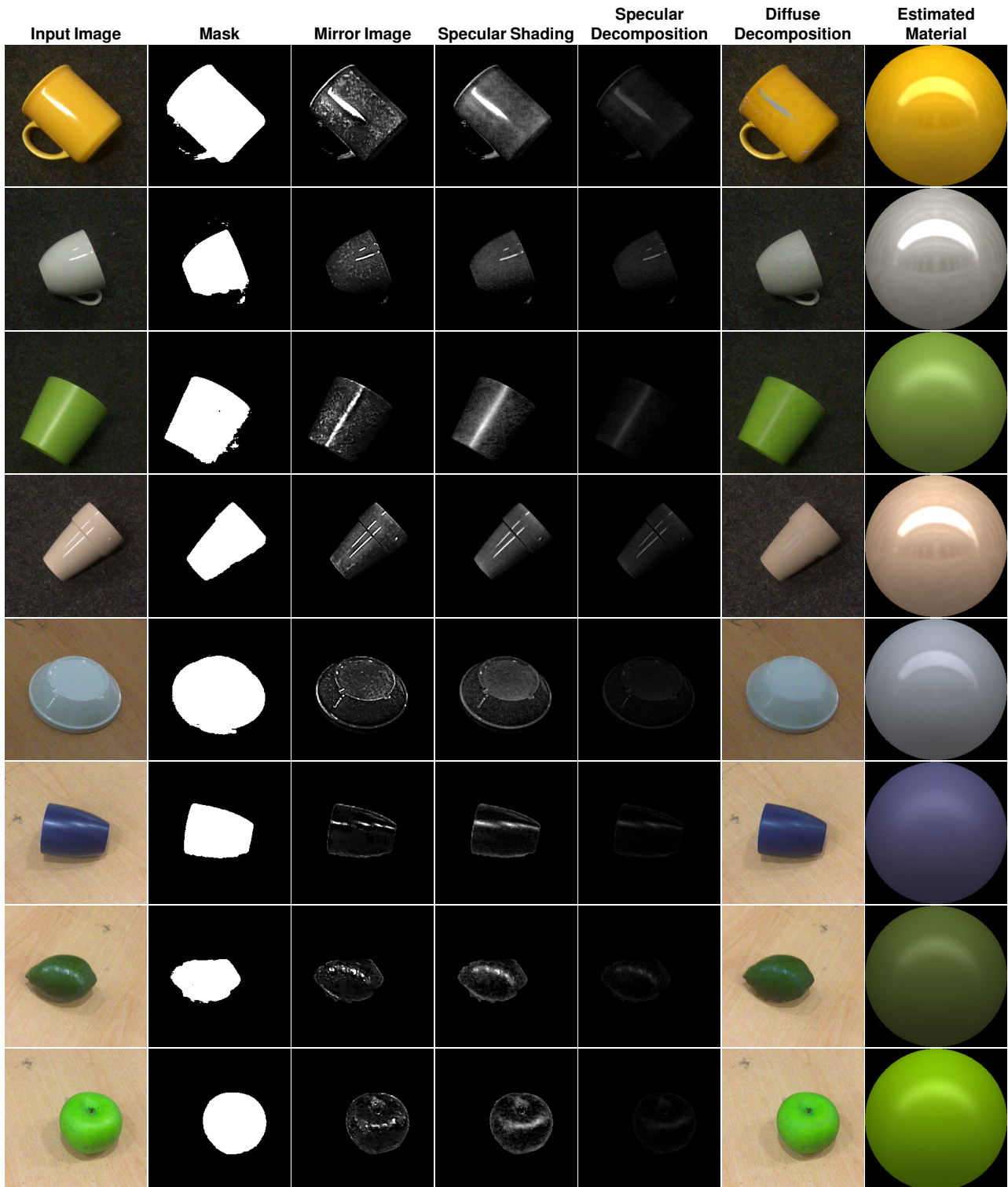
Figure 3. Real-world material estimation results based on a single color input image. Our approach produces high-quality results for a large variety of objects and materials, without manual interaction. Note the high quality of the jointly computed binary segmentation masks.
