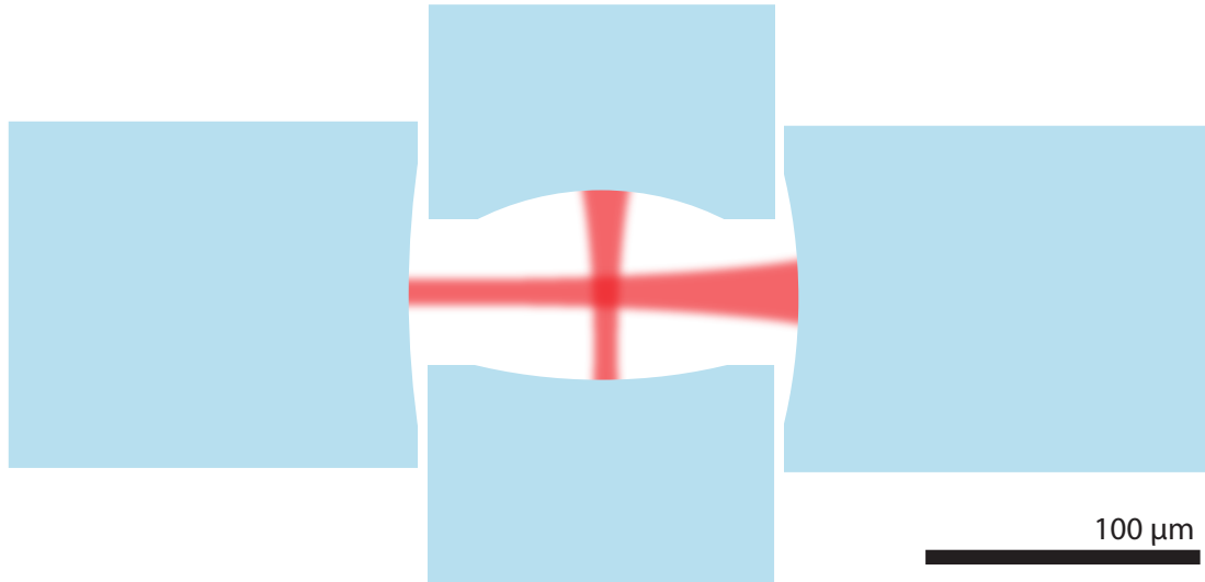
Figure 2.7: The space required for two crossed cavities based on substrates with a diameter of 125\ \mu\text{m} . The short cavity (vertical) has a length of 70\ \mu\text{m} to allow a far off-resonant trap to be focused between the mirrors without excessive scattering. The long cavity (horizontal) has to have a length L > 140\ \mu\text{m} , such that the short cavity fits between its mirrors.
