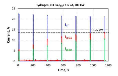
FIGURE 3. 1160s pulse in hydrogen with the 125 kW power limit for the co-extracted electrons on the extraction grid halves
