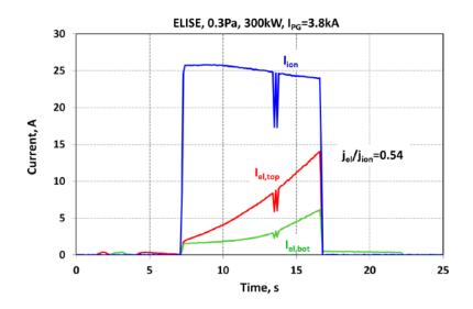
FIGURE 7. 10 s pulse in deuterium with potential rods
