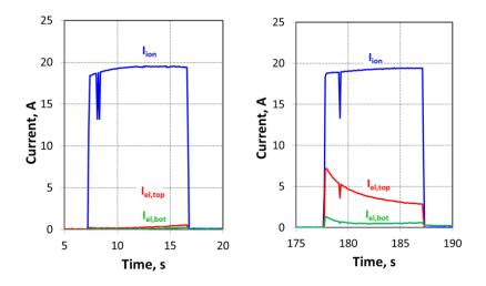
FIGURE 10. First and second beam extraction of the 2700 s pulse in deuterium shown in Fig. 9, the spikes are HV breakdowns
