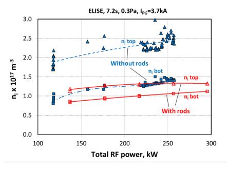
FIGURE 6. Ion density measurements with Langmuir probes close to the top and bottom part of the extraction system with and without potential rods
