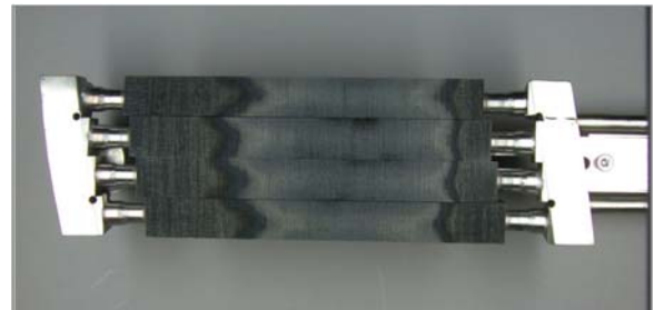
Fig. 11: Picture of the loaded surface of the scraper module prototype after high heat flux cycling and screening tests in GLADIS.
