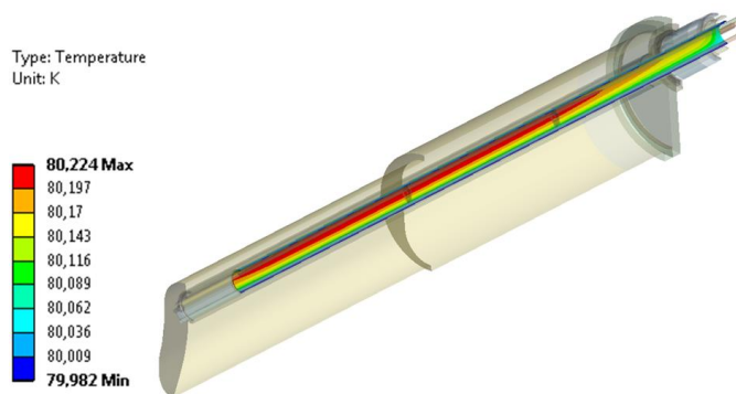
Fig. 5. Temperature distribution of the cryo-shield
