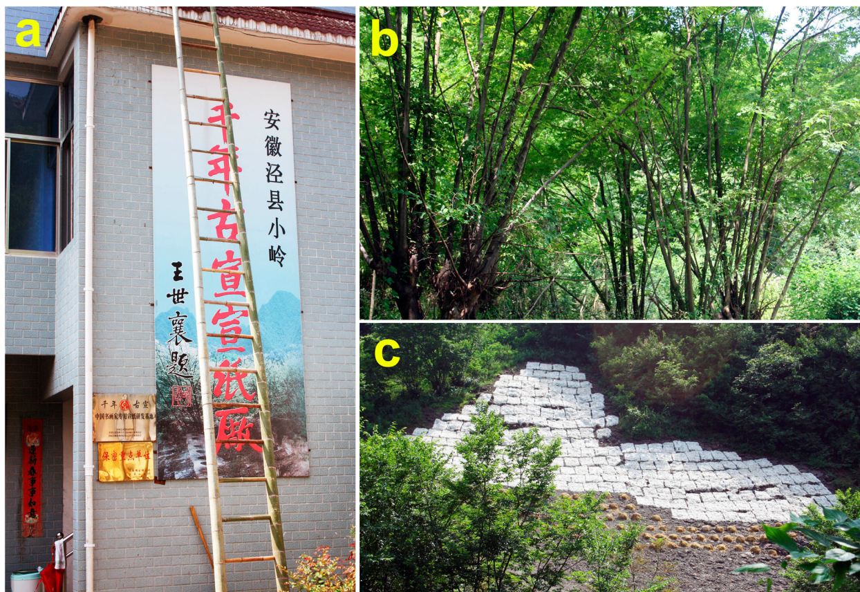
Figure 1. a. the Qian Nian Gu Xuan mill; b, blue sandalwood growing all over the mountains around the mill. The blue sandalwood bark examined in the present study was peeled from one of these trees; c, blue sandalwood bark and rice straw ( liao cao ), both having been cooked, are laid out on weathered rocks on hillsides around the mill, where exposure to the sun allows natural bleaching to occur.
