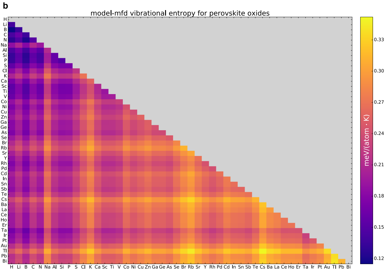
FIG. 3. The predicted vibrational free energy (a) and entropy (b) for perovskite oxides ( ABO_3 ).
