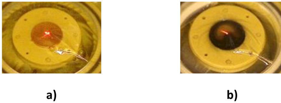
Fig.3.9: The polycrystalline copper electrode a) before and b) after treatment. The different colour of the surface should be noticed (->foil capped).
