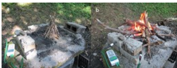
275 Fig 3: Fire pit set up. a) before lighting the fire. b) during the burning.
