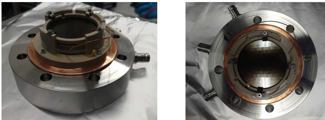
Figure 7.17.: Photograph of the microchannel plate stack for imaging the direct beam and for the grating spectrometer.
