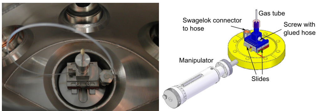
Figure 7.9.: Flange carrying the setup for the HHG. The gastube is built on slides and can be positioned along the NIR beam with a manipulator. The gas is provided via a gas feed through and a hose connecting the feed through and the tube holder.
