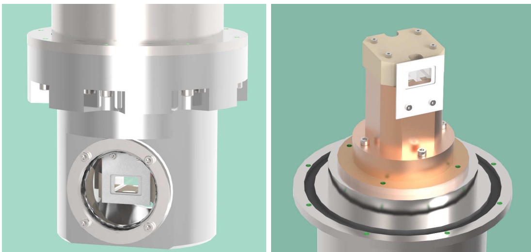
Figure 5.12.: Left: Input window of vacuum chamber for cryogenic cooling of the large aperture PPLN. The symmetric cold finger allows crystals up to a size of 4 cm. Right: Cold finger of the 3.6 cm long large aperture PPLN with the ceramic mask at the input surface.
