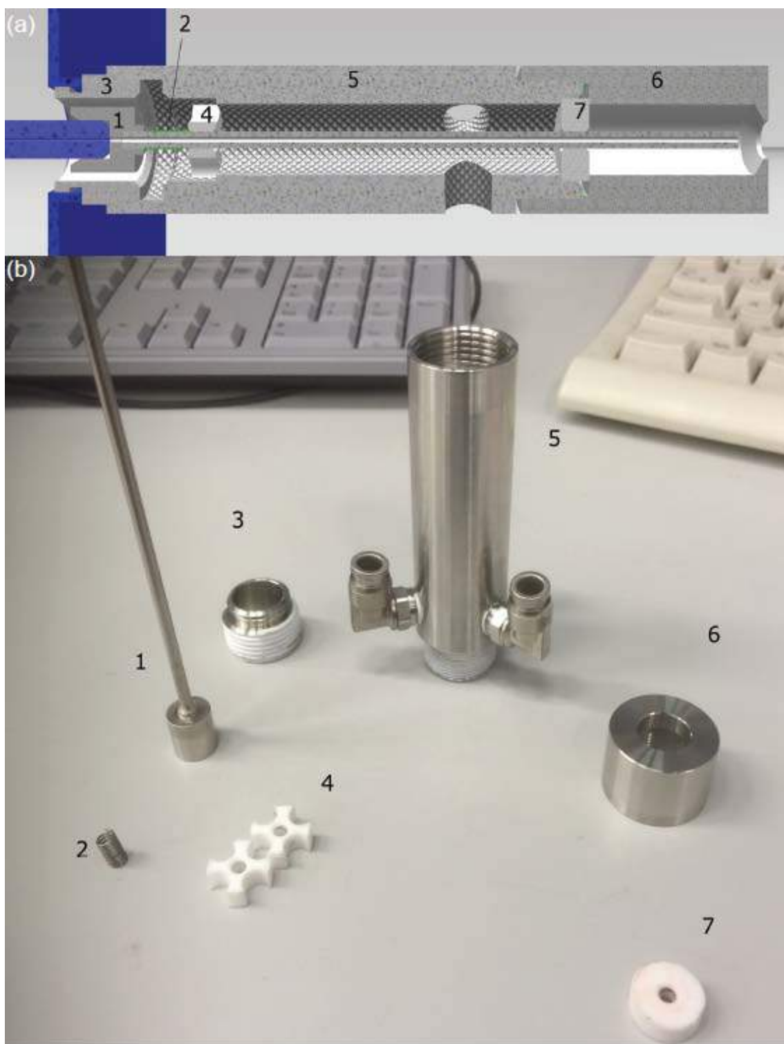
Figure 2.3: (a) cross-section structure and (b) components of gas diverting inlet extension: 1. metal capillary with adapter, 2. tungsten spring, 3. thread adapter, 4. macor spacers, 5. heating sleeve, 6. cap, and 7. macor plug.
