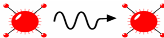
Figure B10.12: Recoil-free emission or absorption of a gamma-ray when the nuclei are in a solid matrix such as a crystal lattice 219
