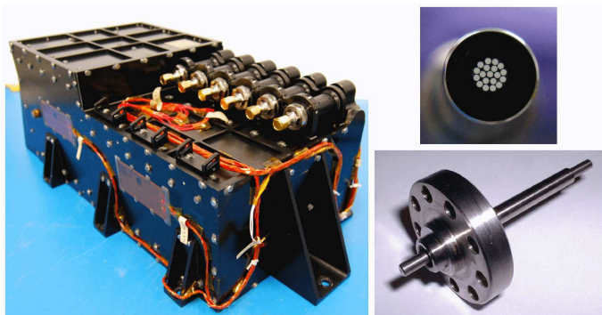
FIG. 1: Left: The flight ULU with external heaters attached. The ends of the six optics barrels are seen temporarily sealed with gold dust caps. Top Right: An end-on view of an FOH with the 19 individual cores visible. Bottom Right: A flight ISUK.
