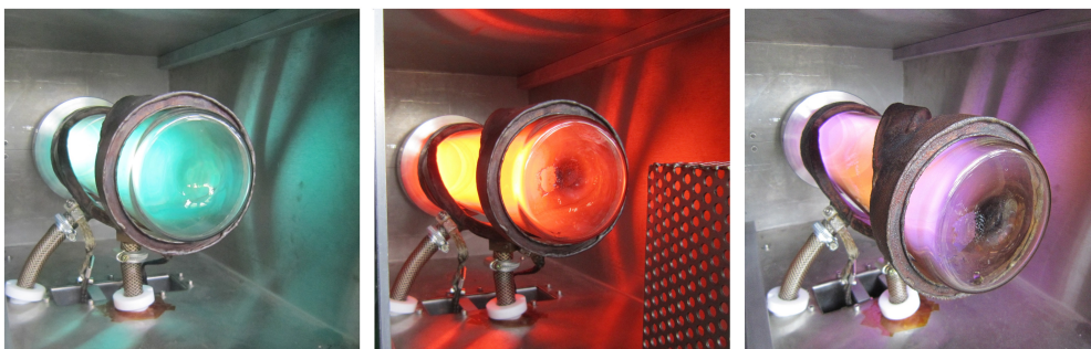
Figure 72 – Different working gases used for plasma generation in VINETA.I. Left image: Helium. Middle image: Neon. Right image: Argon. The plasmas were produced in low power discharges ( < 500 W) with the helicon cell of VINETA.I.
