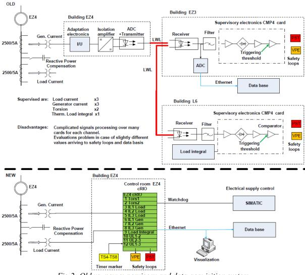
Fig.2: Old vs. new supervisory and data acquisition system
