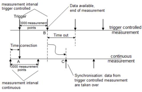
Fig.5: Synchronization of trigger based and continuous measurements
