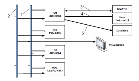
Fig. 3: Supervising hardware architecture. 1- Trigger signal, 2- Network connection between real-time computers and visualization, 3- Bidirectional connection to SIMATIC, 4 – Fiber optic cable for fast control, 5- Network connection to the data base
