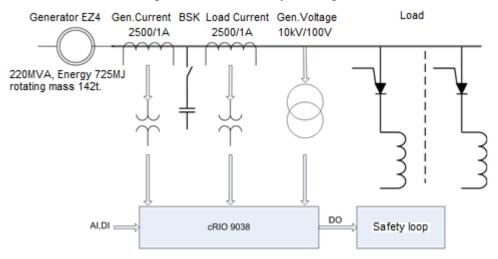
Fig. 4: Supervising system of generator EZ4 with input and output signals
