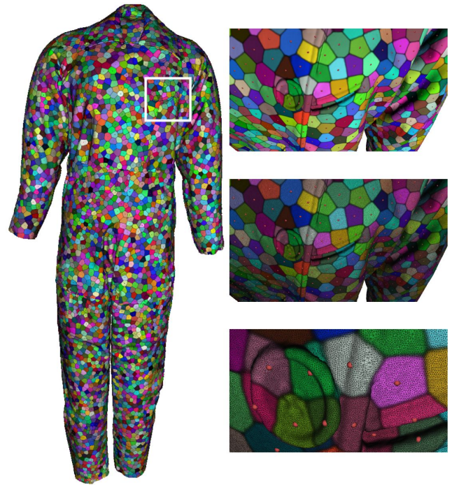
Fig. 14. Earhart's Flight Suit ( 10M\Delta ) with 10 000 seeds, the resulting cells are visualized in different colors. A close-up of the cell distribution (top-row) and the underlying mesh (middle and bottom rows) reveals small scale geometric complexity (pocket fold, button fold) that can successfully be processed with our computationally- and memory efficient approach.
