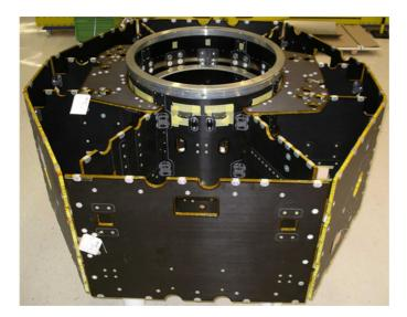
Figure 5. Flight structure of the LISA Pathfinder spacecraft.
