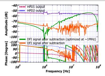
**Figure 6.** The transfer function from the displacement simulator to the interferometer output. The displacement information on the HPD1 and HPD2 is significantly cancelled in the DFI signals
