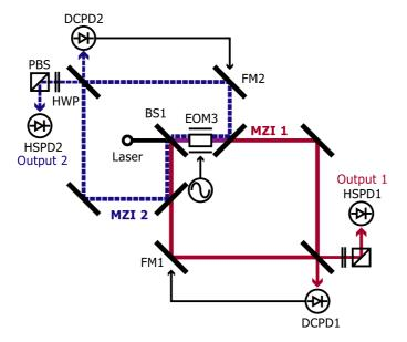
**Figure 5.** Another setup for the partial demonstration of DFI. This is one pair of two independent MZIs sharing beam splitter, which is a part of 3D DFI, to confirm the cancellation of beam splitter displacement.
