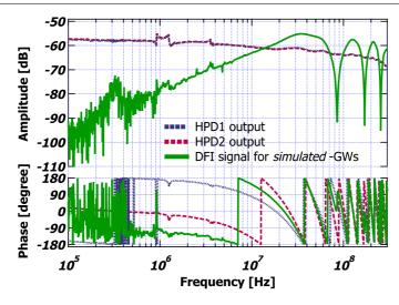
**Figure 4.** The response function to the *simulated*-GW signal. The identical signal subtraction of DFI to the displacement noise gives finite sensitivities to the GW-*like* phase modulations.
