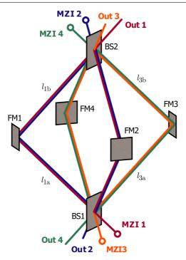
**Figure 1.** A schematic of three-dimensional DFI. The laser light propagates on the ridge line of the octahedron to form four simple MZIs. There are two beam splitters (BS) and four folding mirrors (FM) at the spatially symmetric apexes of the octahedron.
