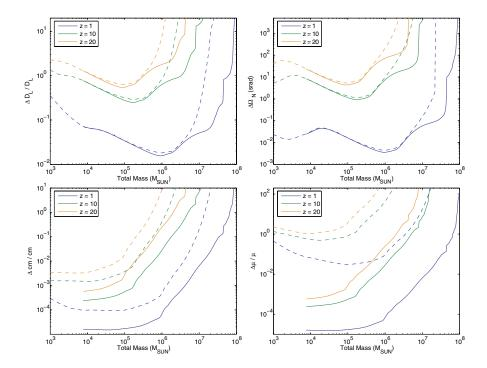
FIG. 6 (color online). Distance measurement error, angular resolution, and mass measurement errors for LISA observations of the final year of equal mass supermassive black hole inspirals. The fiducial sources are at z = 1, 10, and 20. The waveform considered are the FWF at 2PN order (solid lines) and the RWF (dashed lines) with  $\cos\theta_N = -0.6$ ,  $\phi_N = 1$ ,  $\cos\theta_L = 0.2$ ,  $\phi_L = 3$ , and  $\beta = \sigma = 0$ .
