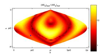
FIG. 10 (color online). Sky map of the gain in angular resolution for LISA observations of the final year of inspirals using FWF versus RWF corresponding to  $m_1 = 10^7 M_{\odot}$ ,  $m_2 = 10^6 M_{\odot}$ , and z = 1. We assume all source have the same orientation  $\cos\theta_L = 0.2$ ,  $\phi_L = 3$ , zero spins  $\beta = \sigma = 0$  and that LISA is at  $\phi_{\text{LISA}} = 0$  at the time of coalescence. The dark blue dot corresponds to  $\cos\theta_N = -0.6$ ,  $\phi_N = 1$ .
