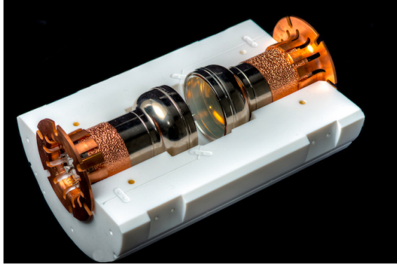
Figure 4.4: Picture of the Teflon block with the two PMTs used for the single phase measurement of ^{83\text{m}}\text{Kr} . Photograph from C. Föhr
