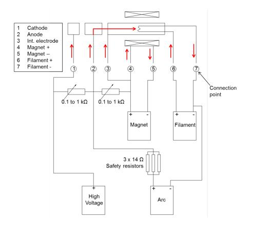
Figure 8: Schematic of the electrical connections of the DuoPIGatron ion source to the power supplies. The red arrows above the connection points represent the direction of the electric current. All connection points as well as the magnet, arc and filament power supplies are set to high voltage by way of the high voltage power supply.
