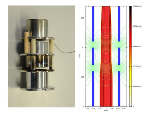
Figure 30: Einzel lens and ion optics simulation of a lens with IBSimu. In this simulation, the central electrode is set to a decelerating potential of +100 V while the first and third electrodes are grounded. A 5 mA beam with an extraction potential of +6 kV was used in this simulation. The lens on the left does not have the same geometry as the simulated lens and is only included for visualization.
