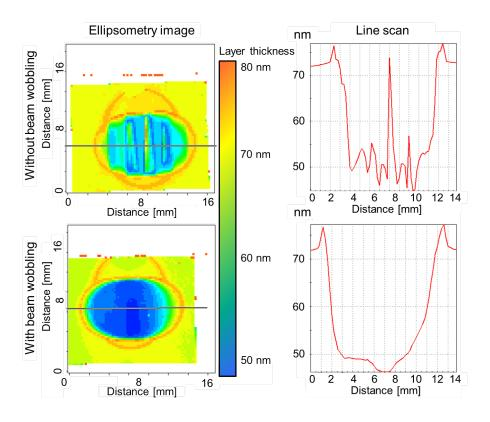
Figure 37: Ellipsometry measurements of the beam footprint at the target obtained by exposing a 70-nm-thick a-C:H layer on Si of a 6 keV  $D_3^+$  beam, when using a Ø 6 mm beam-defining aperture. The images on the left show a 2D pattern of the a-C:H layer erosion. The images on the right are line scans along the line indicated in the left figure. In the lower pair of images, the ion beam was scanned over the beam- defining aperture. For details please refer to the text. (Color online). [23].
