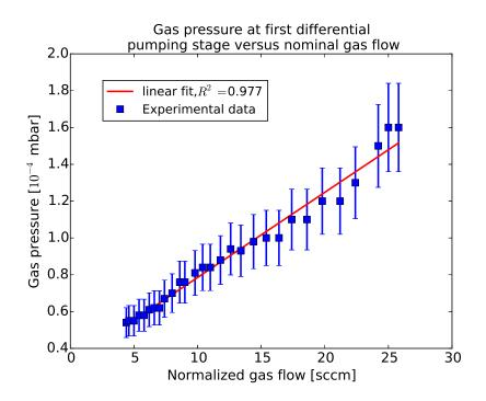
Figure 24: Gas pressure at the first differential pumping stage is plotted versus the flow-controller gas throughput. A linear regression was added, providing a good fit within the experimental error of the gas pressure measurement.
