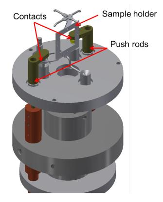
Figure 15: Push rods can be used to press down on the sample holder hind legs, thereby improving the electrical contact between thermocouple contacts and the target.
