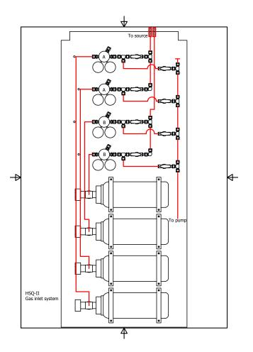
Figure 7: Draft of the gas connection scheme of SIESTA.
