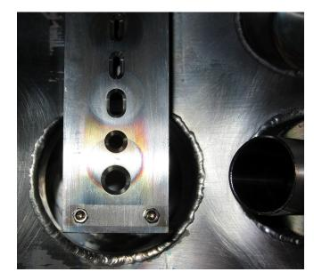
Figure 17: Beam defining aperture in the target chamber. In the picture, the bottom hole is aligned with the ion beam trajectory. The thin plate installed between beam defining aperture and connecting tube to the antechamber is not present. The tube on the right provides a line of sight between the pyrometer and the sample.
