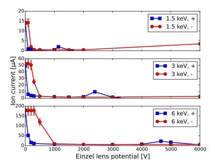
Figure 32: Ion currents measured at the beam-stopper from D beams of 1.5, 3 and 6 keV when operating an einzel lens at the exit of the ion source at varying accelerating and decelerating potentials. Space-charge compensation was lost after applying a modest potential to the lens, as evidenced by the rapid drop in the measured ion current. In no case were ion currents achieved that were larger than without a lens. Lines have been added to guide the eye.
