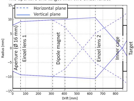
Transfer matrix calculation of the ion optics between Mo aperture and target with two einzel lenses
