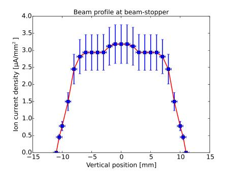
Figure 26: Beam profile at beam-stopper measured with Faraday cup. A line has been added to guide the eye. The ion current density appears to be uniform near the beam axis within the uncertainty of the measurement, with an edge width of approx. 2 mm.
