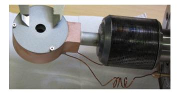
Figure 10: Beam-stopper employed at SIESTA equipped with a faraday cup to measure the ion beam current.
