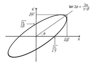
Figure 34: Emittance diagram showing the emittance ellipse parameters, also known as Twiss parameters. For a given position along a beam's trajectory z, the angular distribution of the trajectories along a direction transverse to the nominal path can be described by an ellipse in the (x, x') coordinate system where x denotes the distance along the transverse direction and x' denotes the angle of the beam with regards to z on the xz plane [20]
