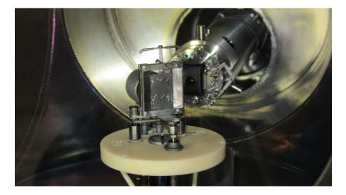
Figure 18: Target holder with sample in TDS chamber. The sample can be biased and can be and heated by a filament located at the backside of the sample, providing electron impact heating. The quadrupole massspectrometer, located behind the target holder, is used to analyze the composition of the gas that is desorbed from the sample.
