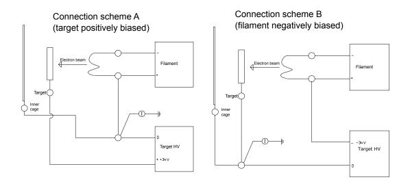
Figure 16: Connection schemes for the target chamber of SIESTA, allowing for the target to be positively biased and the heating filament set to ground potential (A), or conversely for the target to be grounded and the heating filament set to a negative bias (B). In both cases the ion beam impinges on the target from the left, passing through a hole in the grounded inner cage. A current integrator, labeled "T, is used to measure the ion current.
