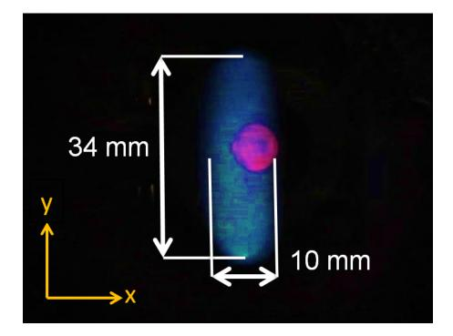
Figure 33: Beam profile of a 10 keV  $D_3^+$  beam on Ce-doped quartz glass 16 cm away from the exit of the dipole magnet. The beam is focused within the magnet in the deflection plane (x), leading to an astigmatic beam with a beam-waist smaller than 10 mm at the quartz glass. The red spot in the middle of the image is light from the ion source that is reflected inside the dipole magnet, and bears no relation to the beam spot.
