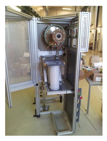
Figure 4: High-voltage cage of the DuoPIGatron ion source. Below the source, the cooling lines coiled into double spirals can be observed.
