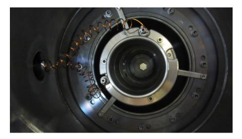
Figure 31: Einzel lens installed in the first differential pumping stage at the exit of the ion source, marked 1st einzel lens in the bird's-eye view of SIESTA (fig. 1).
