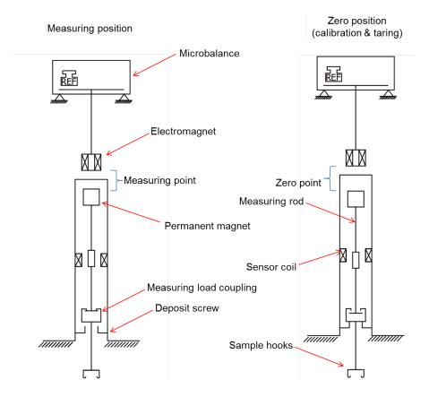
Figure 39: Measurement principle of the Rubotherm magnetic suspension balance. When set to "Zero" mode, the permanent magnet is suspended to the zero point (load not suspended) and the balance is tared and automatically calibrated. When in "Measuring" mode, the permanent magnet is suspended at the measuring point, lifting the sample.
