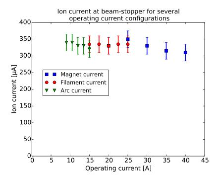
Figure 20: Ion current measured at the beam-stopper with the source magnet, filament and arc set to various operating currents, with all other parameters set to maximize ion current. Within the error of the experimental measurement, no effect of these parameters on the extracted ion current could be observed.
