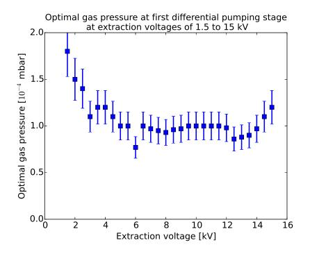
Figure 23: Optimal gas pressure with increasing extraction voltage when using deuterium. For extraction voltages below 4 kV, lower extraction voltages lead to a higher optimal gas pressure. For voltages of or above 4 kV, the pressure optimum is typically in the range of  $10^{-4}$  mbar.
