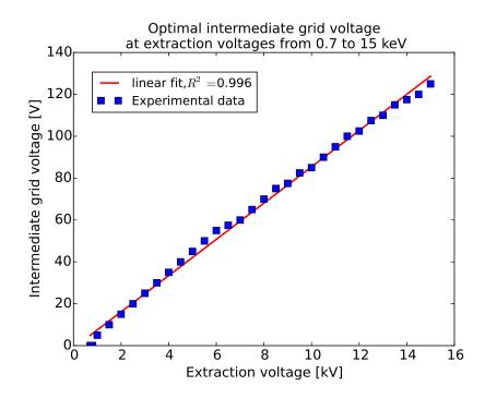
Figure 21: Optimal intermediate grid voltage (negative) for increasing extraction voltages. The error bars for the experimental values are smaller than the size of the markers.
