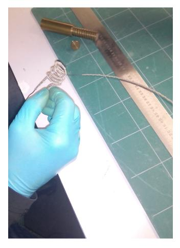
Figure 5: Coiled ion source filament before coating. In the background, the grooved brass cylinder used to coil the filament and an uncoiled tantalum filament, already wrapped in a nickel mesh, can be seen.
