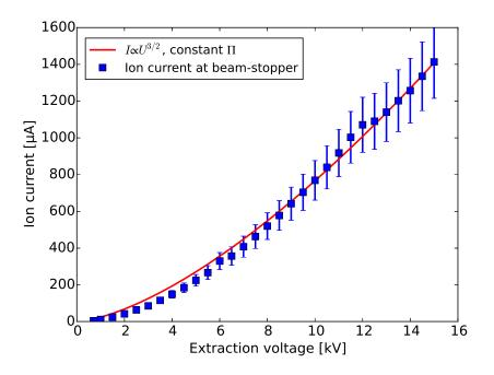
Figure 19: Ion current measured at the beam-stopper with increasing extraction voltage, fitted with a curve of constant perveance as described in eq. 2 [9]. The increase in the size of the error bars for ion currents above 1 mA is due to a change in the measurement range of the current integrator.
