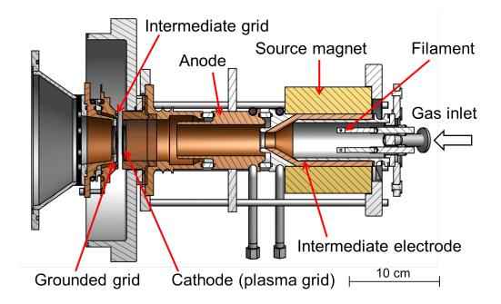
Figure 3: Half-section view of the DuoPIGatron ion source. No filament is in place in the figure.
