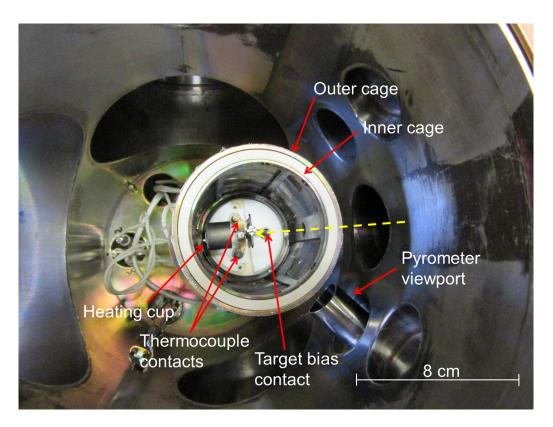
Figure 13: Top view of target chamber interior showing the double cage, pyrometer viewport, heating cup and target holder with thermocouple and target bias contacts. The beam defining aperture is absent. The beam direction is from right to left as indicated by the yellow dashed arrow.
