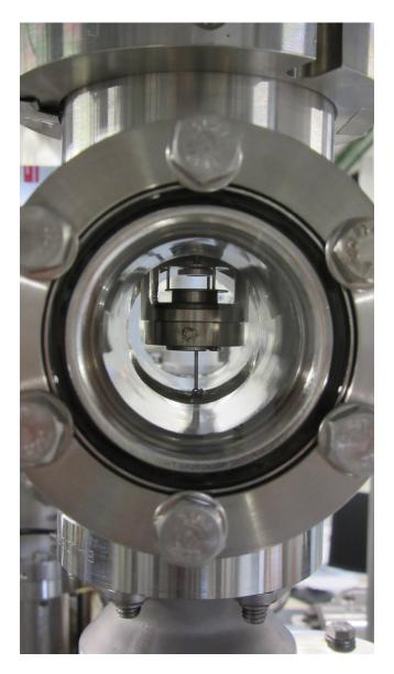
Figure 40: Microbalance measuring load coupling observed through CF40 viewport above the target chamber.
