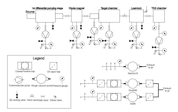
Figure 9: Schematic of the vacuum system of SIESTA.
