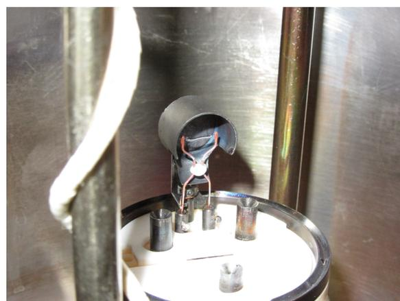
Figure 14: Target platform with heating filament, with (left) and without target (right). The two hind legs of the target holder are connected to a type-K thermocouple. The front leg is connected to a power supply which sets the bias of the sample. The heating cup is electrically connected to the heating filament. The hooks situated on top of the target holder are used to weigh the sample and to transport it between target chamber, load-lock and TDS chamber.
