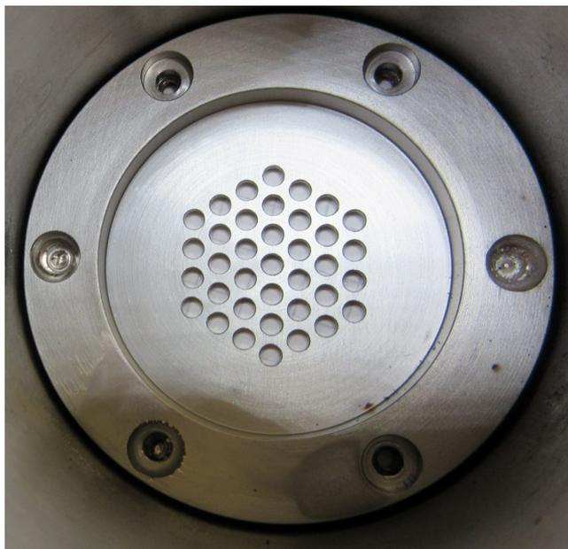
Figure 6: Ion source extraction grid with partly-melted steel screws. The screw heads have either melted or have broken off due to thermal stresses.
