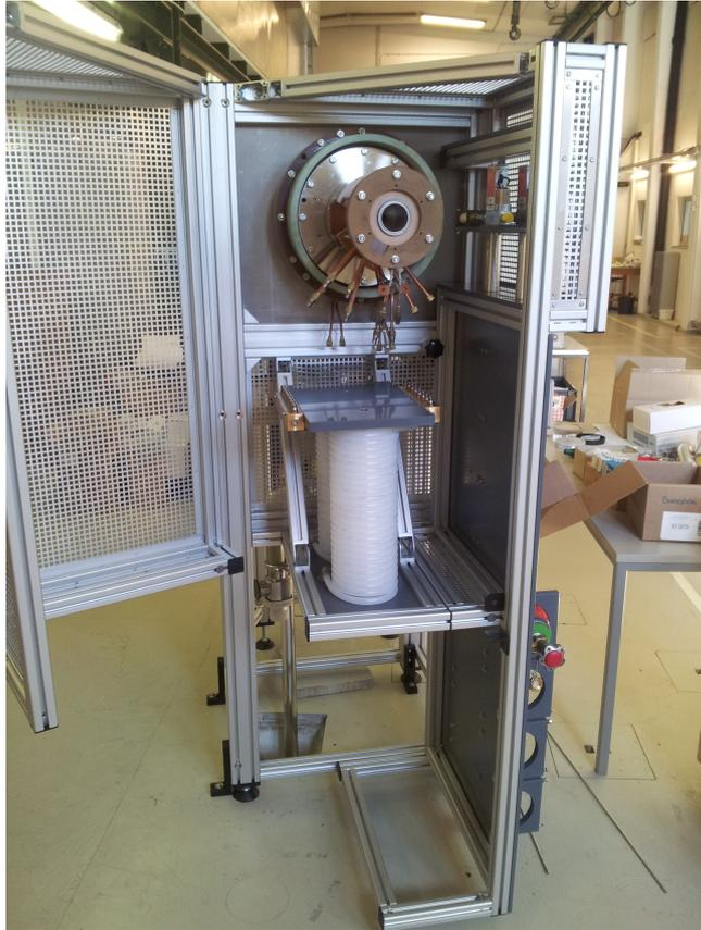
Figure 4: High-voltage cage of the DuoPIGatron ion source. Below the source, the cooling lines coiled into double spirals can be observed.
