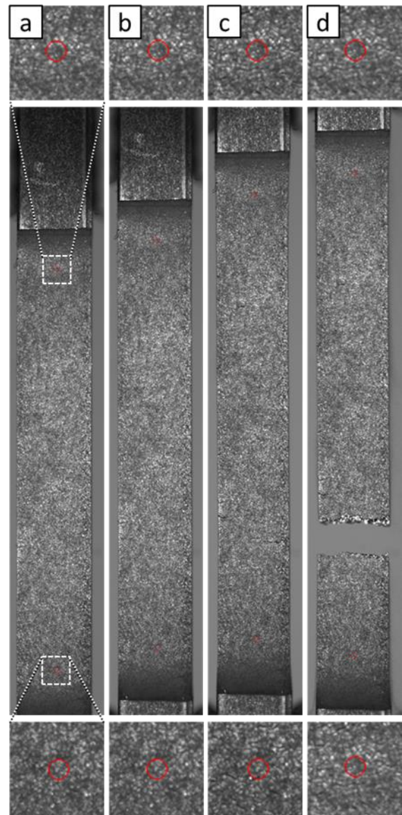
Figure 1 Example images as used by DIC, a) Strain = 0% (initial), b) Strain = 1.43%, c) Strain = 10.7% (last frame before fracture), d) First frame after fracture
