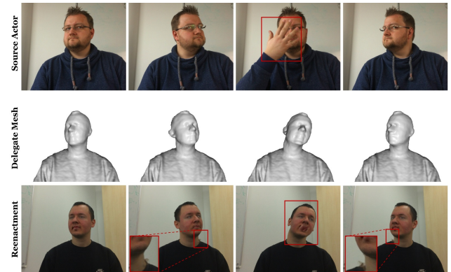
Fig. 17. Limitation: Strong head rotations or occlusions in the input stream of the source actor lead to distortions in the reenactment result.
