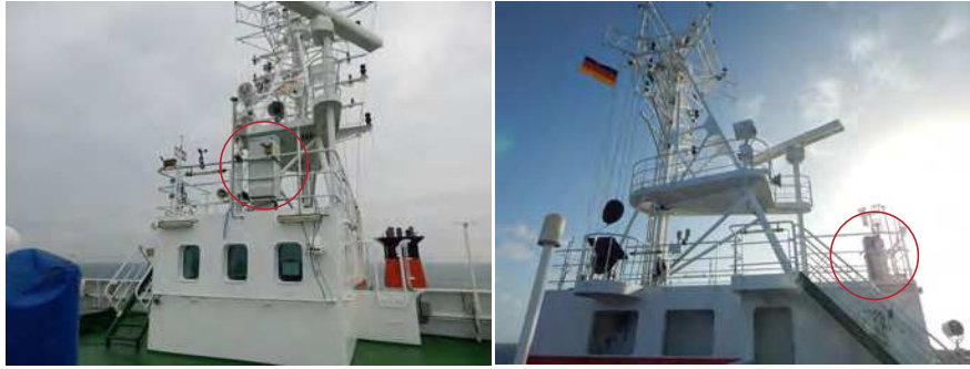
Figure 23: Ceilometer during MSM 68/2. Shown are photos of the instrument from different angles.
