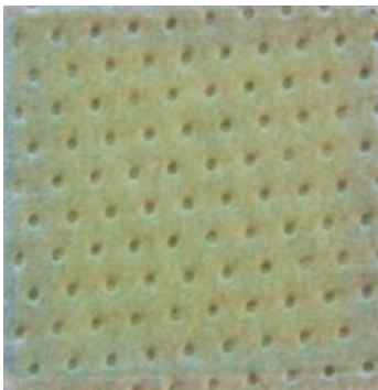
Figure S32. Picture of the films of 20 nm obtained by sublimation onto glass substrates using the Na[Dy(5,7-ClIq) 4 ] ( 2(Dy) ) complexes. Note that the substrate is placed on top of a paper towel after being deposited in the ultra-high vacuum system in the glovebox.
