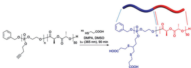
Fig. 6 Synthetic route to silver-bearing degradable polymeric nanoparticles: post-polymerization modification of alkyne-functionalized PPE- b -PLLA via thiol-yne "click" reaction to prepare anionic amphiphilic diblock copolymer, reproduced from ref. 322 with permission from the American Chemical Society, Copyright 2017.
