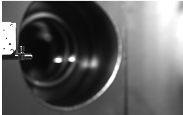
FIGURE 5.11: Picture of the injector mounted in the vacuum chamber recorded for the size calibration. The illumination is done by a halogen lamp in the vessel. The resolution of the picture is 1280 \text{ px} \times 800 \text{ px} .
