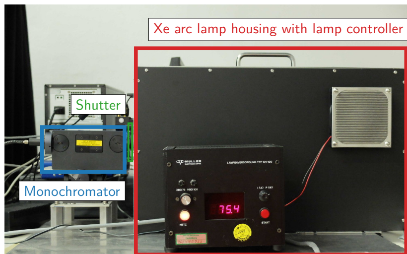
Figure 2.2 Light source setup outside the dark box. The Xe arc lamp is positioned within a special fan-cooled housing to avoid eye contact with the produced UV light and to decrease the generated heat. Exiting light is focused into a monochromator whose entrance slit can be closed with a shutter mounted on a flipper device. By means of an optical fibre the light is guided into a dark box.
