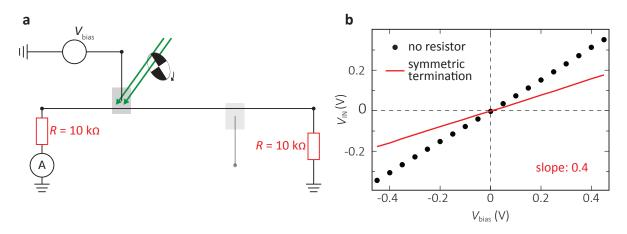
Fig. S12 | Symmetric termination of the central microstrip. a, Schematic representation of the experimental setup with a symmetric 10 k $\Omega$  termination. b, Measured signal compared to a measurement with a termination on one side only.
