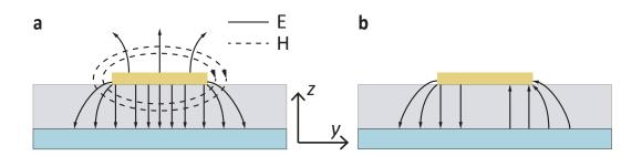
**Fig. S8** | **Electric field distribution for microstrip modes. a**, Fundamental mode. **b**, First higher order quasi-TE<sub>10</sub> mode, which cannot be excited in this experiment, where the distance between backplane (blue) and the microstrip as well as the width of the microstrip are both much smaller than the guided signal wavelength (0.3  $\mu$ m and 6  $\mu$ m << 100  $\mu$ m - 300  $\mu$ m ).
