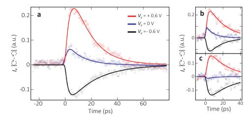
**Fig. S17** | **Raw Hall current data including a zero source-drain voltage background signal. a**,  $I_x[\bigcirc - \bigcirc]$  data from Fig. 3a (main text) including the zero source-drain voltage background signal. **b**, and **c**,  $I_x[\bigcirc - \bigcirc]$  taken after two different thermal cycles.
