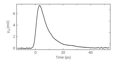
**Fig. S14** | **Pump-probe signal.** The generator switch is biased with  $V_{\text{bias}} = 5$  V and sampled by a second switch 600 µm away. The curve is scaled to report the amplitude of the input signal into the LIA after being amplified with  $A_{\text{TIA}} = 2 \cdot 10^9$  V/A.
