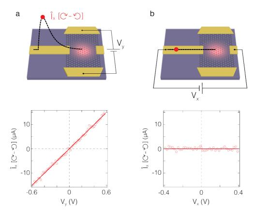
**Fig. 3** | **Helicity-dependent current behavior under different source-drain voltage geometries.** The peak of the helicity-dependent current  $\hat{I}_x$  [ $\bigcirc - \bigcirc$ ] measured as a function of **a**, transverse source-drain voltage V<sub>y</sub> and **b**, longitudinal source-drain voltage V<sub>x</sub>. The graphene Fermi level was gated to the Dirac point (E<sub>F</sub> = 0). Solids lines are linear fits.
