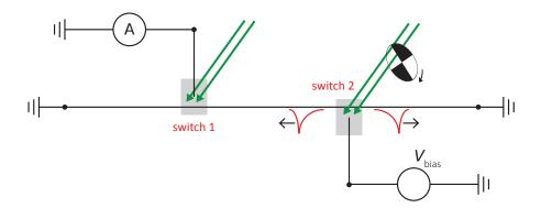
**Fig. S13** | **Pump-probe measurement setup.** Switch 2 (right) is held under a DC voltage bias and used as a generator for short pulses. By varying the time delay between triggering the detector switch 1 (left) and switch 2, the temporal profile of the pulse is recorded.
