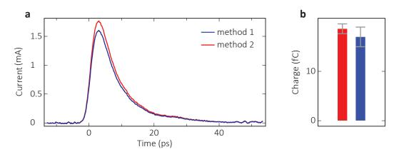
Fig. S15 | Comparison of the two methods to quantitatively characterize the transient current in the microstrip. a, Reconstructed current profile according to method 1 (blue) and method 2 (red).
