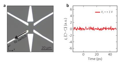
**Fig. S19** | **Test measurements on a device without a graphene flake. a**, Optical microscopy image of a device without a graphene flake. The device has the same geometry discussed in section S5. **b**, Helicity dependent currents  $I_x[\bigcirc - \bigcirc]$  measured at the left switch.
