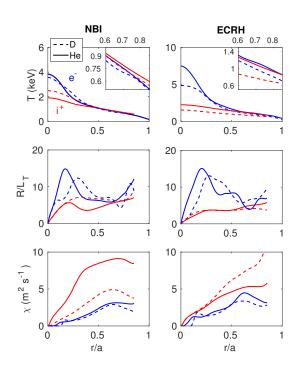
Figure 2: Electron and ion temperature profiles for the highest NBI (left)/ECRH (right) heated plasmas. The normalised temperature gradients  $R/L_T$  and power balance heat diffusivities  $\chi$  are also shown against r/a.
