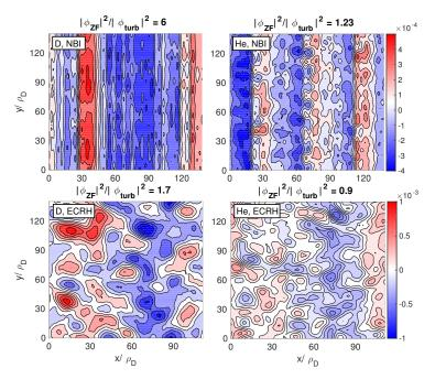
Figure 3: Contours of the perturbed electrostatic potential in the plane perpendicular to the magnetic field at the low field side, computed from local non-linear gyrokinetic simulations of the deuterium NBI and ECRH cases (left panels) at r/a = 0.3 and r/a = 0.5 respectively. The same simulations have been carried out by changing only the main ion species to He (right panels).
