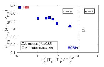
Figure 4: Normalised ratios of the highest linear growth rates of the ETG and ITG instabilities versus the electron to ion collisional thermal coupling strength for He plasmas. Low density cases are represented by open symbols.
