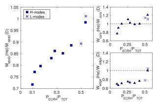
Figure 1: Ratio of the helium to deuterium measured total plasma stored energy against the ratio of ECRH over the total heating power (left panel). Core and edge contributions to the stored energies (right panels).
