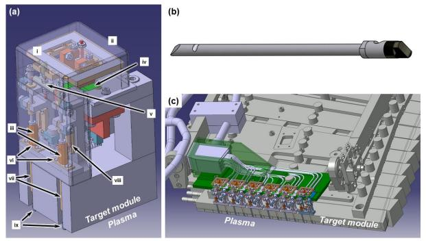
Figure 1. (a) CAD model of two probes and one drive unit with labels indicating the different components described in the text. (b) Replaceable probe. (c) View of 12 probes and 6 drive units on a target module, as well as the cable conduit system.
