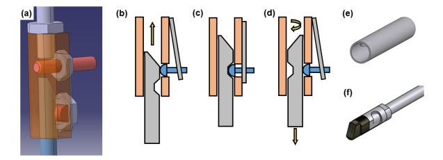
Figure 3: (a) Detail from the CAD model of the probe and fixation. (b) Conceptual illustration of the insertion of the probe into the fixation. (c) The inserted position, after the probe has snapped into place. (d) Removal of the probe. (e) Removal tool. (f) Detail of probe tip showing interface to removal tool.
