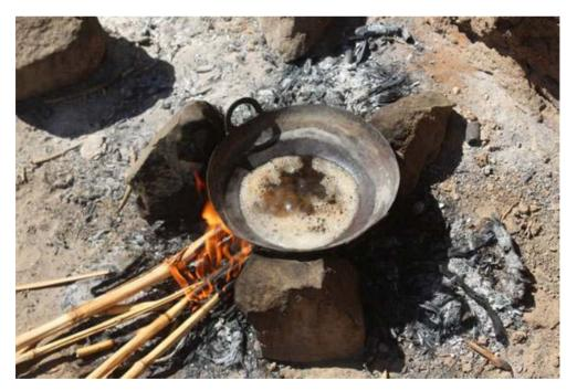
THE BITTER POTASH SOLUTION IS BROUGHT TO A BOIL. WHEN FOAM FORMS ON ITS SURFACE, THE INTENSITY OF FIRE MUST BE REDUCED IN ORDER TO PREVENT THE LIQUID FROM OVERFLOWING. PHOTO BY LAURENCE DOUNY
