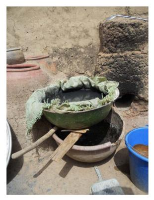
THE fILTERING OF ASHES, LIXIVIATION OR SLOW PERCOLATION PROCESS IS CARRIED OUT WITH TWO CONTAINERS: ONE THAT IS PERFORATED AND IN WHICH THE ASHES AND THE WATER ARE POURED AND A SECOND CONTAINER, HERE A CLAY POT PLACED UNDERNEATH, THAT COLLECTS THE FILTRATE. PHOTO BY LAURENCE DOUNY
