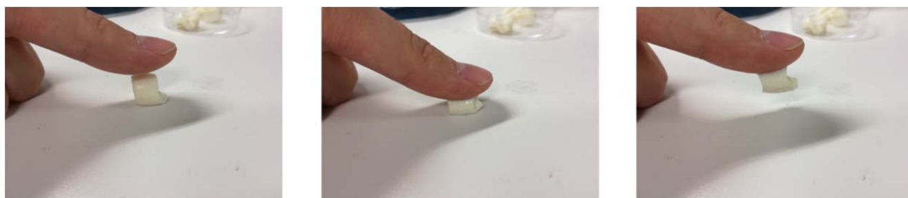
Figure S8. Gentle compression on 2 wt.% g-CN-AHPA hydrogel and its adhesion to finger.
