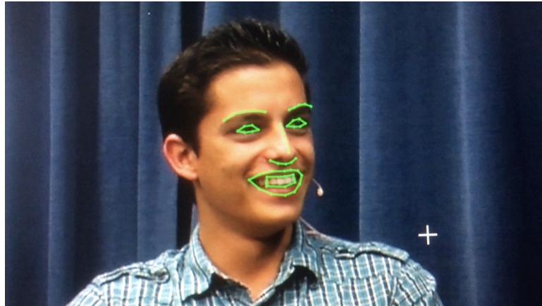
Figure 1. Still image from facial motion tracking-based blink detection. The green little dots on the green lines represent the pixels being tracked over time. A blink was automatically detected when the distance between dots on the upper lid and dots on the lower lid was reduced beyond a predefined threshold.
